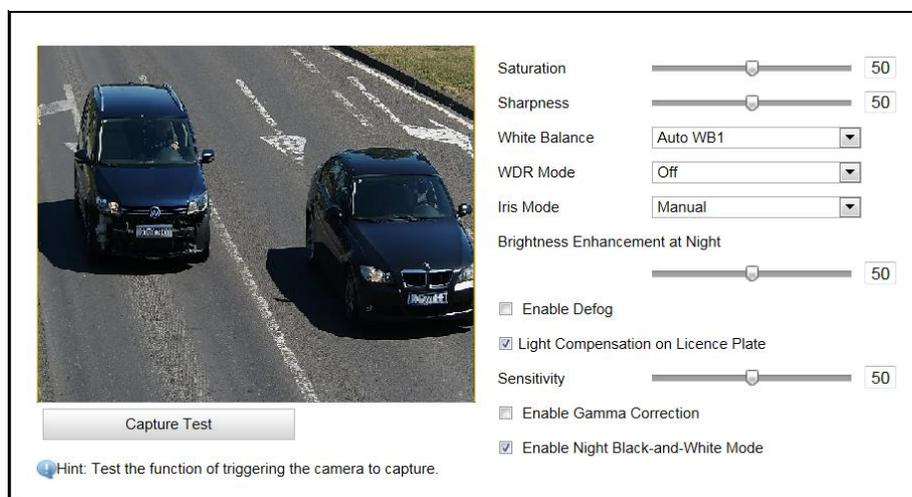
Figure 12-1 General Parameters Configuration
